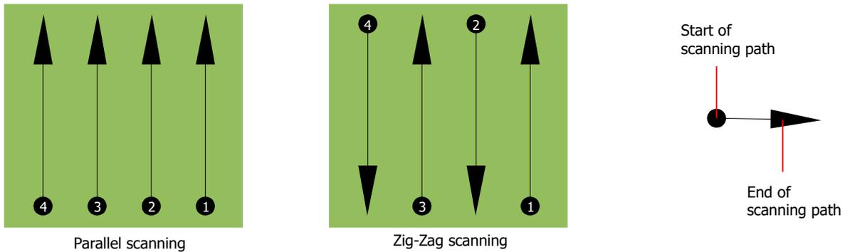
Figure 8.2: Scan modes to measure an area
